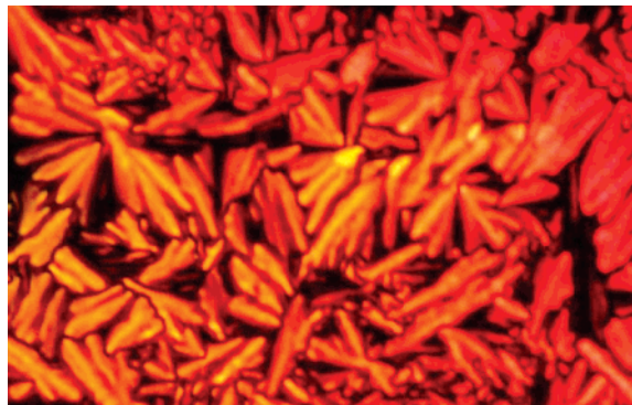
Figure 2. Uranyl complex of 2b forming a liquid crystal, as seen through photomicrography. The mesophase is observed here at 124 °C and is stable between 108 and 135 °C.
